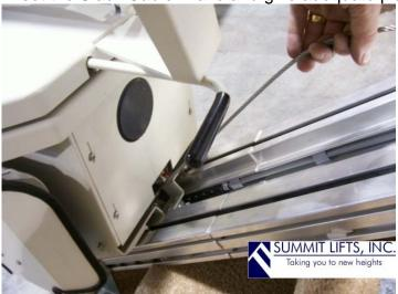
3) Remove the trailing cord from the adhesive clip closest to the chain.
