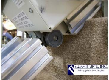
15) Remove the wheels and replace with new ones.
